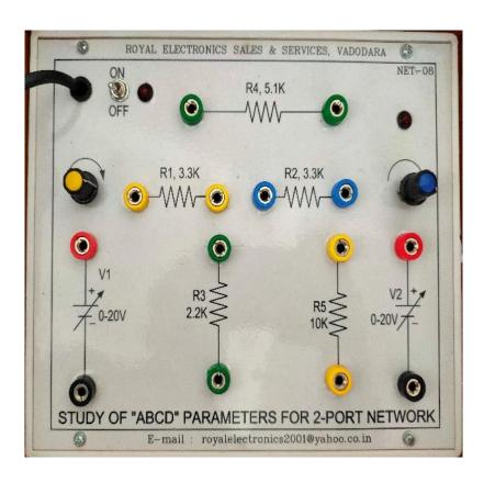
Basic Details: - Study of ABCD Parameters for 2-port network circuit can be performed.
