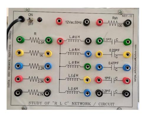
Basic Details: - Study of RLC network circuit can be performed
