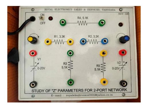
Basic Details: - To study the Z-parameter for 2-port network circuit
